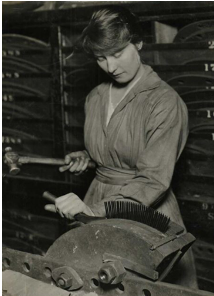
Forming Up Blading, WWI, Parsons Engineering Works, Newcastle-Upon-Tyne, C. Tyne and Wear Archive.
