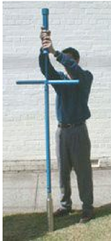
Figure 7.1. Example of a slide hammer driven, two-inch diameter core sampling device.
